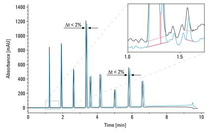
The standard delay volume configuration allows you to run not only RRLC but also conventional HPLC methods without compromising performance or changing chromatographic patterns.
