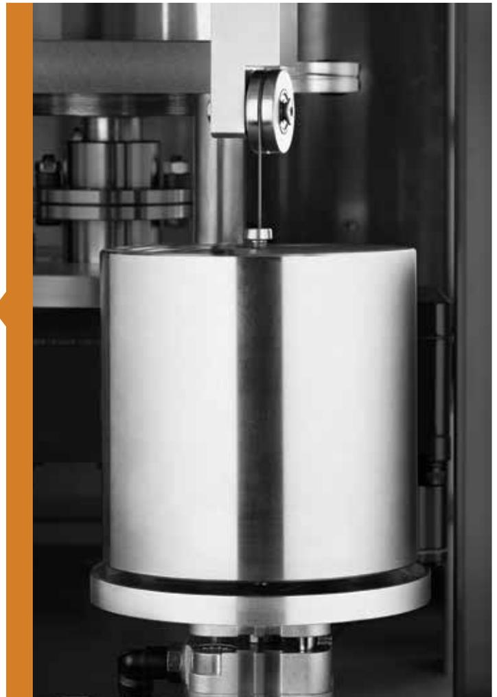
Integrated Torque Calibration
