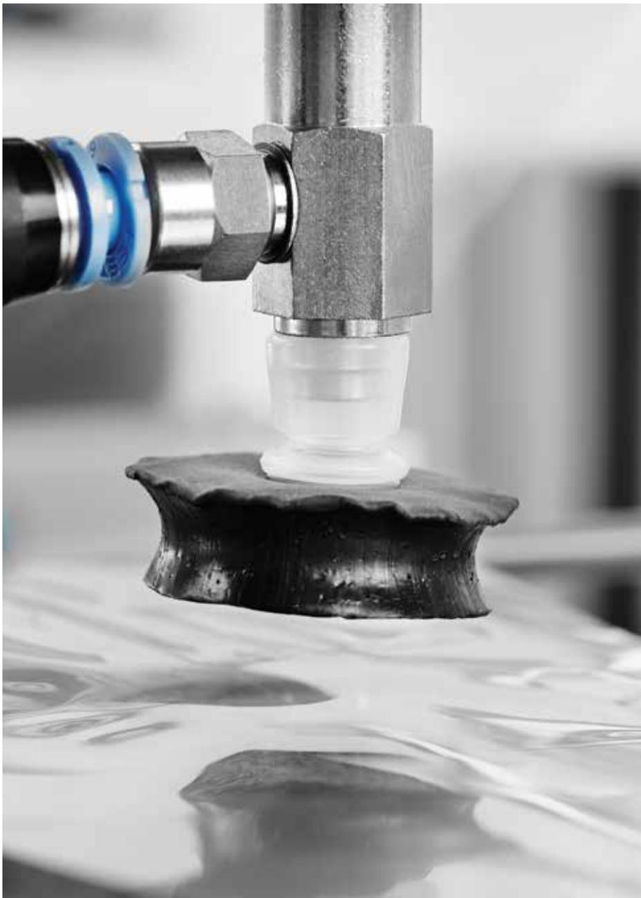
Samples are moved from the autosampler tray to the test position using a suction transfer system. This system is highly tolerant of non-ideal sample geometries, so uncured rubber from many sources can be used. Samples are loaded on a carousel and more specimens may be added while another test is in progress, allowing for uninterrupted productivity.\*
