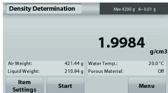
Once the necessary weights have been determined, the density of the sample is displayed in  $\text{g/cm}^3$  (along with the weight in air, weight in water) on the Application screen.
