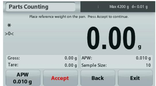
Place the reference weight on the pan, then touch **Accept** to capture the value, the screen shows number of pcs.
