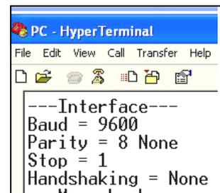
Use RS232 Interface Commands (Section 9.6.1) to control the balance from a PC.
