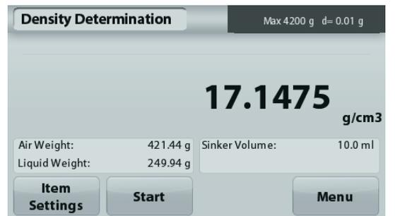
**4.5.5 Measuring the Density of Porous Material Using Oil**
