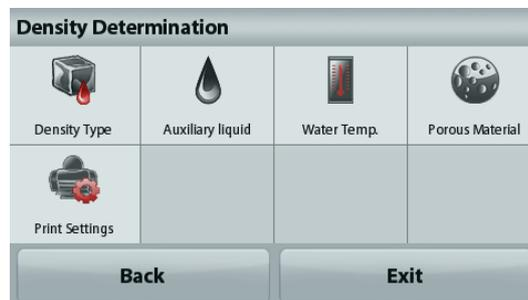
To adjust the water temperature value, touch the **Water Temp.** button.
