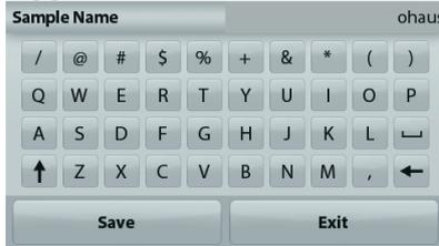
Key in the desired sample name and press Save to save the name and return to weighing home screen.
