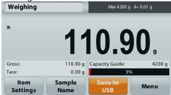
**Notes:** The first time a USB flash drive is connected to the balance there might be some delay time before the button **Save to USB** works. This is due to that the balance is creating the necessary folders on the USB flash drive where the data will be stored. The Density Determination and Check Weighing applications do not have a Save to USB button.
