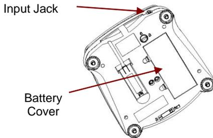
Connect the AC Adapter plug to the input jack.
