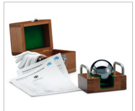
1 kg silicon sphere YDR1000SIC
