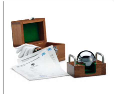
1 kg silicon sphere YDR1000SIC
