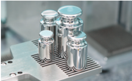
Comb-type weight grabber with 4 weights
