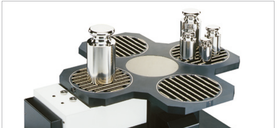
Subdivision weighing on CCE1000S-L | CCE1000U-L | CCE2000S-L
