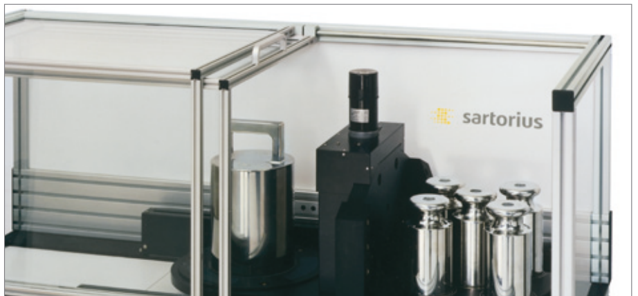
Comparison of a weight with a group of mass standards using the CCE50001S-L
