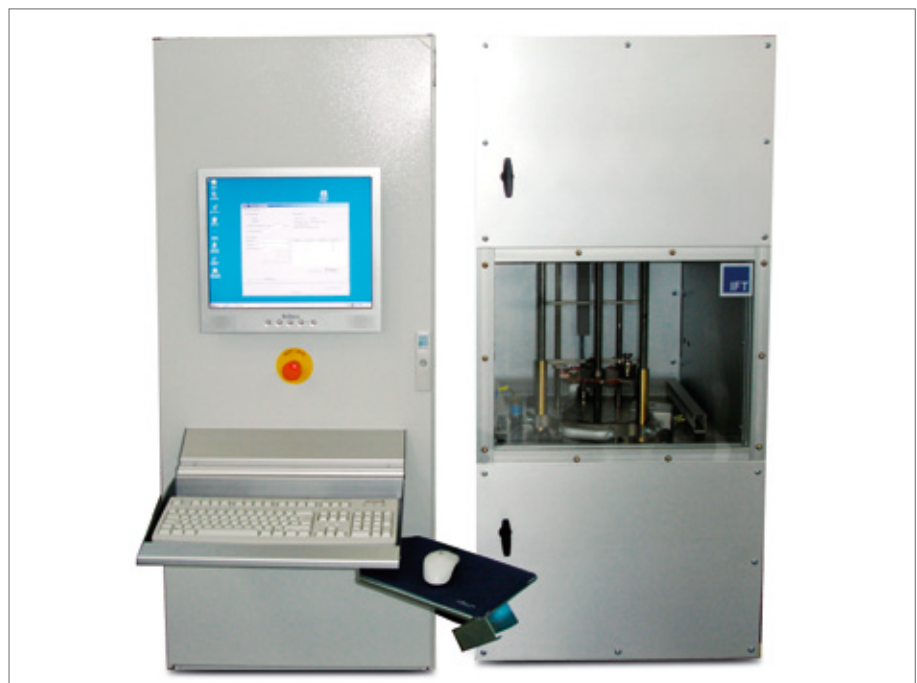
Volume Comparator VD1005|VL1005 (VD 2×9 load alternator positions)
