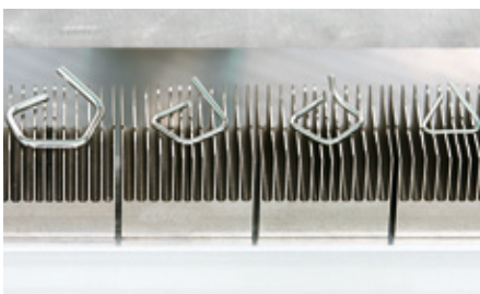
Detail of the magazine for CCR10-1000 (1 mg – 10 g)
