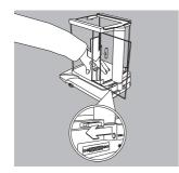
• Secure the draft shield by pressing lightly on the draft shield base and moving the sliding lock device to the left
