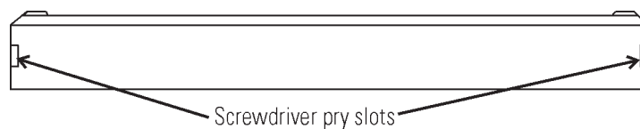
Figure 5-9. Front Cover Plate Below the Door
