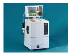
Order no. Vacuum Pump V-700 advanced Completely enclosed, guiet chemically resistant PTFE diaphragm pump with a transparent window heads and with a flow rate of 1.8 m<sup>3</sup>/h and an ultimate vacuum of under 10 mbar, including a vacuum controller V-850.
