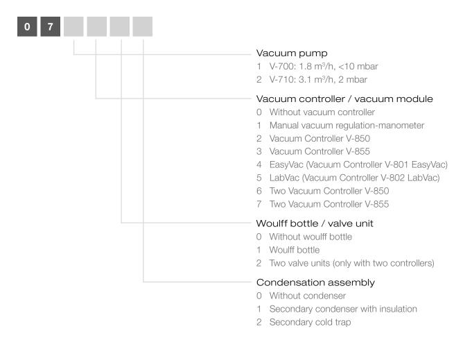
If you order one pump with two Vacuum Controller (0716XX, 0717XX) you need to choose two valve units with it (071X20). The woulff bottle is not needed for this configuration. If you order a pump with one, or without controller (0711XX - 0715XX) you can choose, if with or without a woulff bottle. Although, with a controller it is recommended. In combination with a controller the valve units are not needed.
