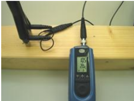
Figure 4-1 Measuring across the fibre direction with M 20
