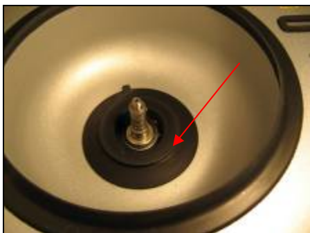
Plastic debris in the centrifuge.
