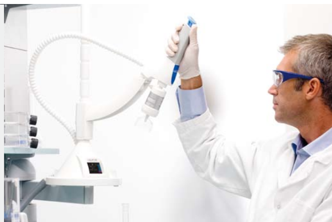
Move the POD dispenser from the arm and just press the plunger.
