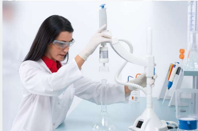
Adjust the POD arm to accommodate glassware.
