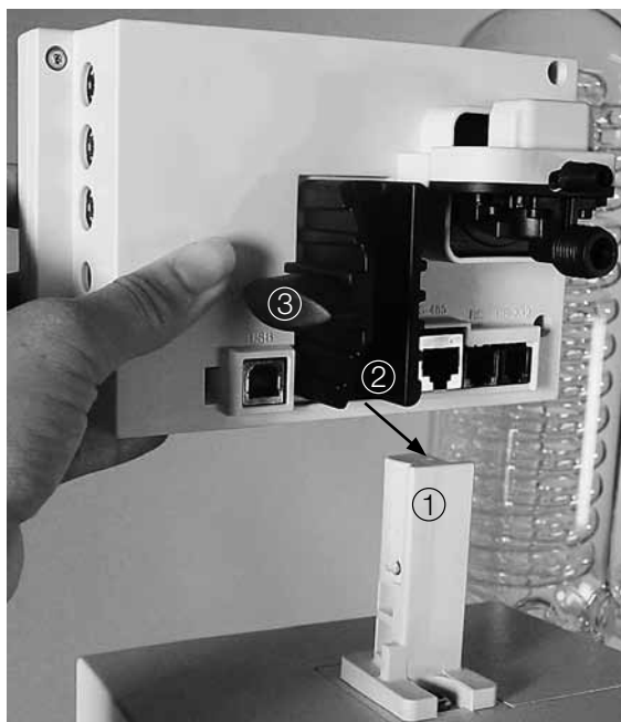
Fig. 5.12: Installing the vacuum controller
