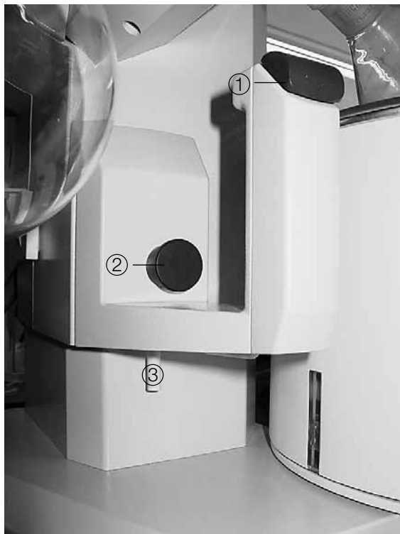
Fig. 6.4: Lowering and raising the evaporating flask
