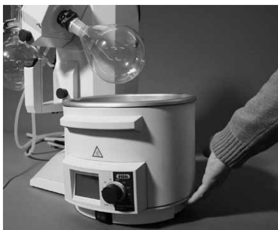
Fig. 5.1: Moving the heating bath
