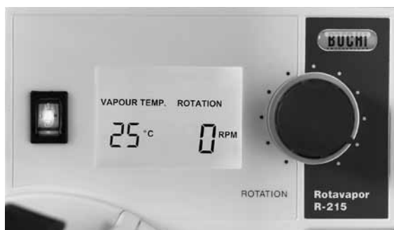
Fig. 4.8: Vapor temperature display at the R-215
