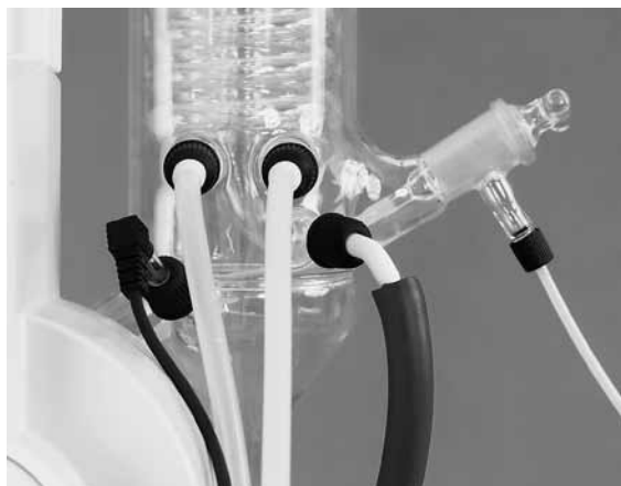
Fig. 5.9: Cooling water tubes
