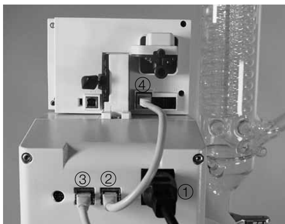
Fig. 5.13: Cable connections to the Rotavapor
