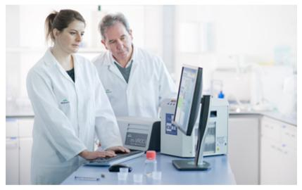
The m-VROCi microfluidic rheometry principle provides high resolution viscosity measurements to ultra-high shear rates with small sample volumes
