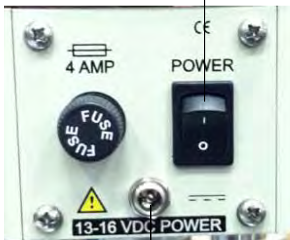
Input Connector: 13 - 16 VDC Power Inlet / Emergency Disconnect Device
