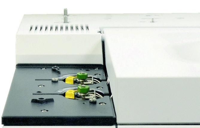
Samples can be injected into the inlets by an automatic sampling device (such as an Agilent Automatic Liquid Sampler or Agilent Headspace Sampler), or by hand using a syringe.
