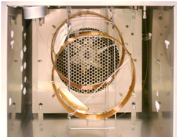
Agilent also offers Low Thermal Mass (LTM) columns. These columns mount in a special oven door and provide fast heat-up and cooldown cycles.
