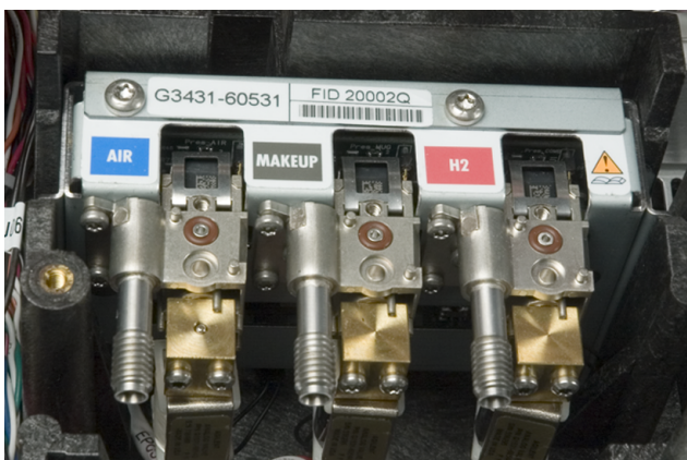
Figure 11 Detector flow module
