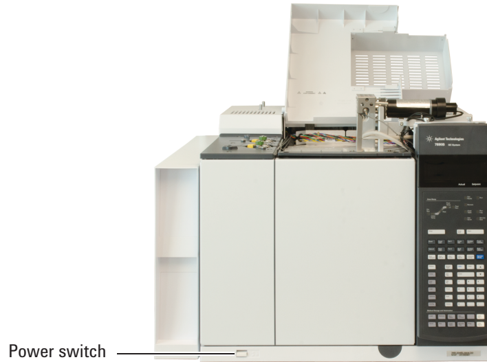
Figure 4 Power switch location
