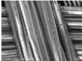
High Vacuum mode without metal coating : Image distortion due to surface charging.
