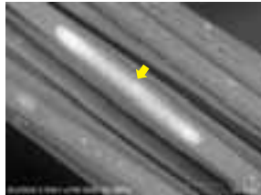
Observation without metal coating : Clearer material contrast of Ti (arrowed) at low vacuum mode.
