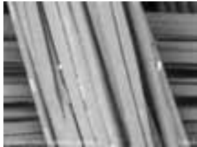
Low Vacuum mode without metal coating : Less specimen surface charging.
