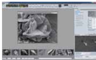
Single image display (800 x 600 pixels) Good for finding observation target or focus adjustment.
