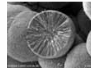
Sample : Titanium Oxide Particle Accelerating Voltage :3kV, Magnification : x15,000, Without metal coating Sample : Courtesy of Prof.Masato Kakiyama,Tohoku University
