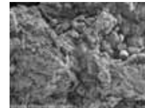
Sample : Polyvinyl Alcohol Accelerating Voltage : 3kV, Vacuum: 60Pa, Magnification : x1,000, Detector: Ultra Variable- Pressure Detector, Without metal coating
