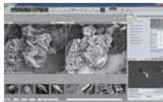
Dual image display (800 x 600 pixels x 2) Two different signal of live images are displayed simultaneously. This allows effective image comparison like the SE/UVD for surface info or BSE compositional image.
