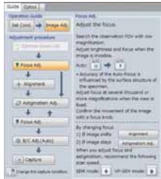
Guide screen for focus adjustment
