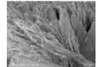
Sample : Gold-Isocyanide Complex Accelerating Voltage : 1.5kV, Magnification : x2,100 Without metal coating
