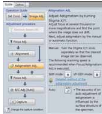
Guide screen for astigmatism correction
