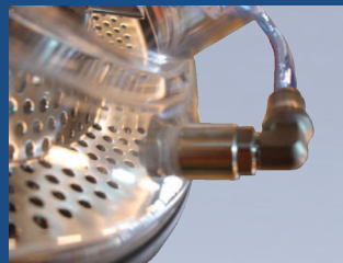
Dust agitation system for optimum dedusting
