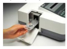
The new source lamp assembly makes lamp changing extremely easy. There is no need to remove the instrument top cover - simply snap out the lamp compartment lid, slide out the lamp assembly and replace with a new one. No lamp adjustment is necessary since the lamps are pre-aligned, and a motorized lamp mirror optimizes for maximum energy throughput during calibration.
