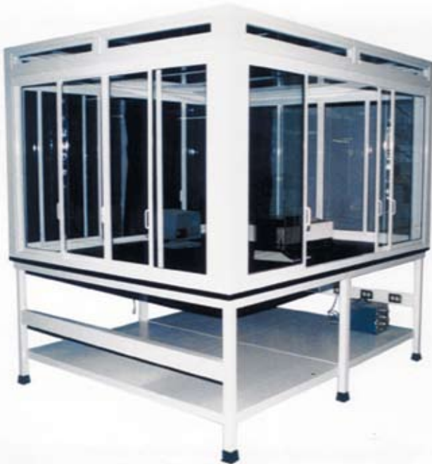
ROBOTIC VENTED ENCLOSURE 8'W x 6'D x 4'H has clear viewing and access on all sides. Fumes are exhausted through a clear slotted ceiling baffle allowing surrounding light to enter.
