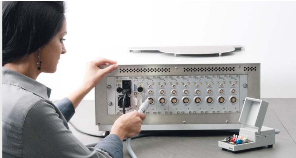
DEA laboratory version with 8 DEA modules (backside view) plus adaptor box for connection to implantable sensors
