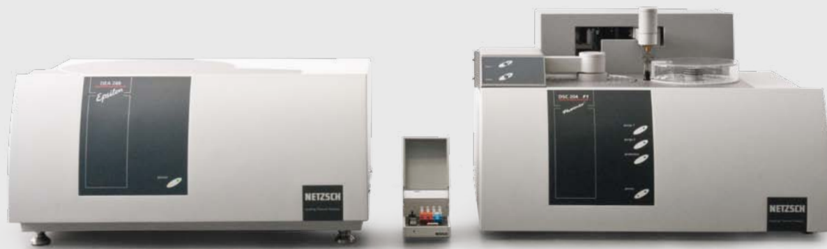
Sensible testing configuration for analyzing curing reactions: DEA 288 Epsilon (laboratory version, left), adaptor box, DSC 204 F1 Phoenix® with ASC (right)
