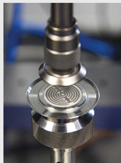
DEA 288 Epsilon with reusable TMS™ sensor (comb sensor with 0.5-mm electrode spacing), integrated in a MARS III Rheometer (plate-plate, gap >0.6 mm)
