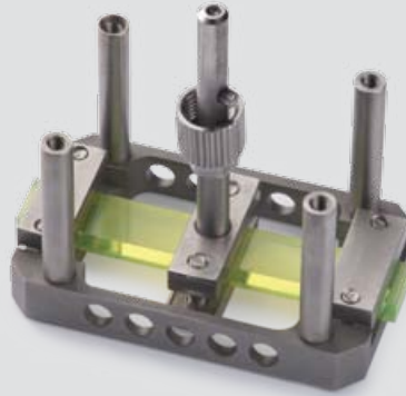
Sample holder for dual cantilever bending
