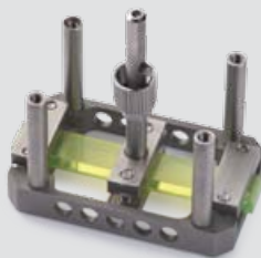
Sample holder for single/dual cantilever
