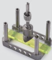
Sample holder for 3-point bending
