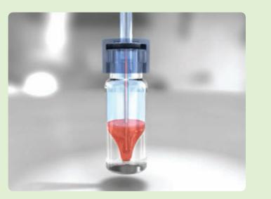
The ekspert nanoLC 400 autosampler uses a dual needle-design and advanced washing capabilities enable the use of extremely limited sample volumes and limits carryover. Automatic vial bottom-sensing ensures minimal sample waste and helps to avoid clogged needles.
