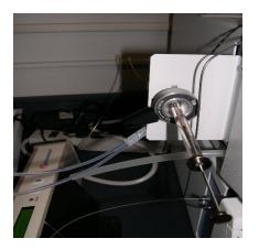
This loads the sample into the sample loop. Remove the syringe. Now rotate the injection valve lever clockwise until it stops, **this injects the sample into the column and starts the software.** Once the sample is injected into the column wait 30 seconds, then rotate the sample valve lever counter-clockwise back to the load position. Rinse the syringe with D.I water.
