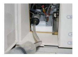
Rotate injection valve clockwise to the inject position so the valve handle is at 10 o'clock.
