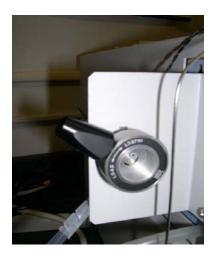
Using the syringe, pull mobile phase through the injection valve and into the syringe. Observe the tubing connecting the mobile phase bottles to the valve, pull enough liquid through the valve to remove any air bubbles in the tubing.
