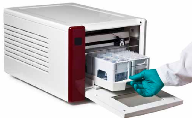
Fig 8. Fraction Collector F9-C holds cassettes for a variety of tubes from 3 to 50 ml as well as 24-, 48-, and 96- deep-well plates.
