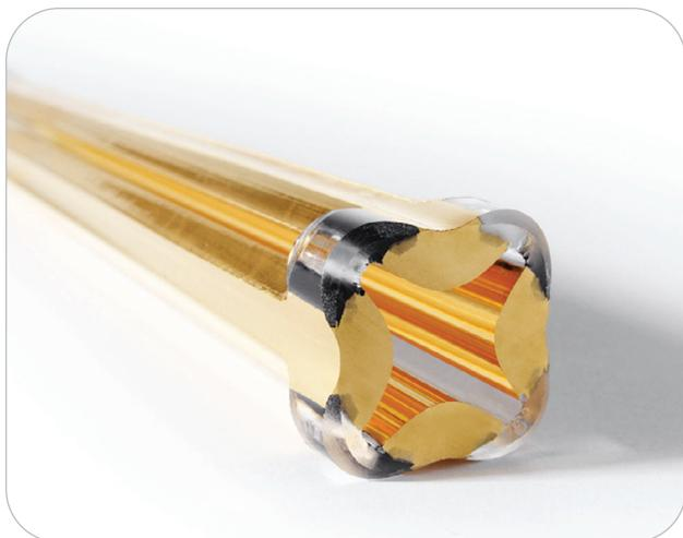
The true hyperbolic quartz structure offers extremely low thermal expansion, and exhibits excellent dimensional stability. The unique design results in lower field errors versus round rod quadrupoles, as well as excellent resolution and mass axis stability, regardless of laboratory temperature fluctuations.
