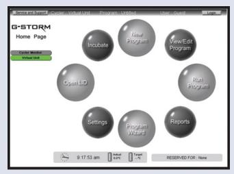
GS2's "Home Page" is central to the control of the cycler's various functions. Select the various options, including Program Wizard, New Program, Run Program, on the touch-screen and let the software take you through a logical process that enables you to do what you want to do in easy, simple to follow steps.
