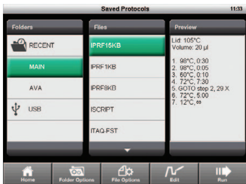
Saved Protocols screen showing the preinstalled library of standard protocols in the MAIN folder.
