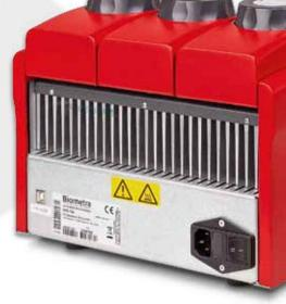
Two air inlets are located at the bottom of the TProfessional TRIO. Inside the housing the air is efficiently transmitted by vents to all heat emitting parts. The air leaves the instrument at the rear.
