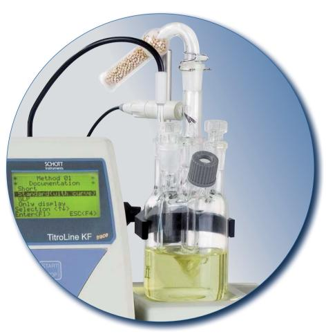
The titration vessels are hermetically sealed and avoid the penetration of moisture extensively (low drift!). The removable glass vessel from the TitroLine KF is available in two sizes and it is easy to clean. For the TitroLine KF *trace* are to be used two different glass vessels with 3 and 5 openings. Both have a very low drift.
