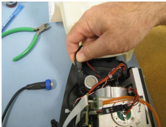
**Figure 20.** Disconnecting the USB cable
