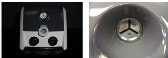
**Figure 14.** Humidity indicator on rear of Cary 630 FTIR (left), and close-up (right)
