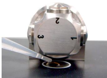
**Figure 10.** Placing sample on the DialPath accessory sample mounting window
