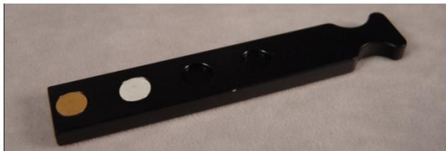
**Figure 11.** Diffuse Reflectance sample holder
