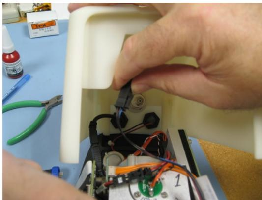
**Figure 19.** Disengaging the power harness
