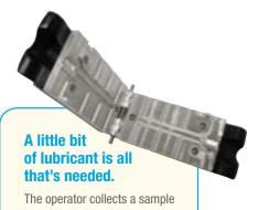
into a 60µL disposable pipette and dispenses the sample into the top of the split-cell capillary channel. The sample then traverses the channel and is accurately timed by the internal processor, reporting kinematic viscosity.
