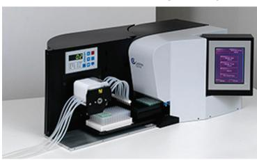
The BioFill is an automated platform for dispensing liquids into screw-cap vials in combination with automated decapping and recapping. The BioFill is based on automatically decapping, dispensing cell suspensions and other liquids into microtubes and recapping the tubes in a 24, 48, or 96 rack SBS-1 footprint.
