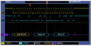
Triggering on a specific data packet going across an l<sup>2</sup>C bus. The yellow waveform is clock and the blue waveform is data. A bus waveform provides decoded packet content including Start, Address, Read/Write, Data, and Stop.
