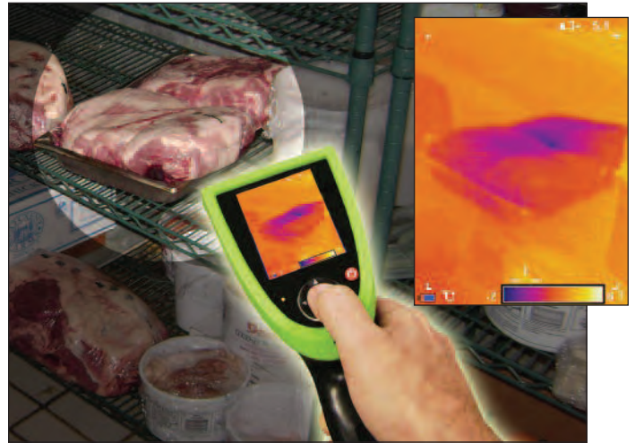
OSXL160 shown measuring temperature of food stored in a walk-in cooler.
