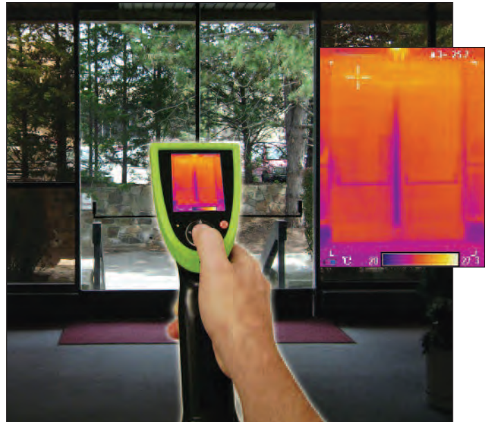
OSXL160 shown measuring thermal leakage around a doorway.
