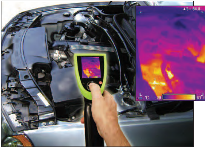
OSXL160 shown measuring an engine's surface temperature.
