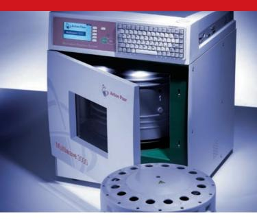
The Multiwave 3000 is a modular platform for microwave-assisted sample preparation. The compatibility of system accessories and a high degree of flexibility meet individual analytical and economic conditions. Sophisticated sensor and vessel technologies solve even the most demanding tasks.
