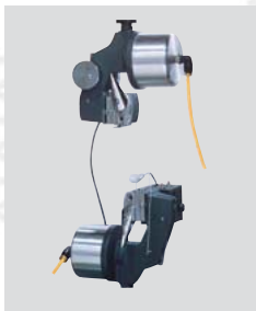
Grips of pneumatic capstan type
