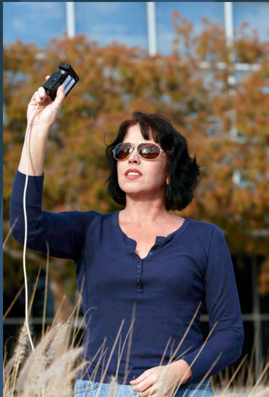
Solar Irradiance Measurements with USB2000+ Miniature Spectrometer
