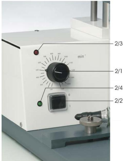
Abb. 2: Adjustment of the piston rotation speed
