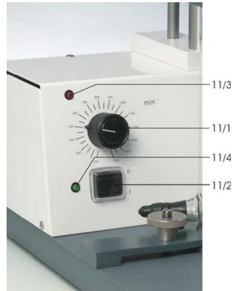
Abb. 11: Setting the rotation speed
