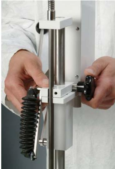
Abb. 10: Setting the normal position of the carriage
