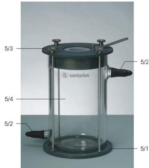
Abb. 5: Cooling vessel
