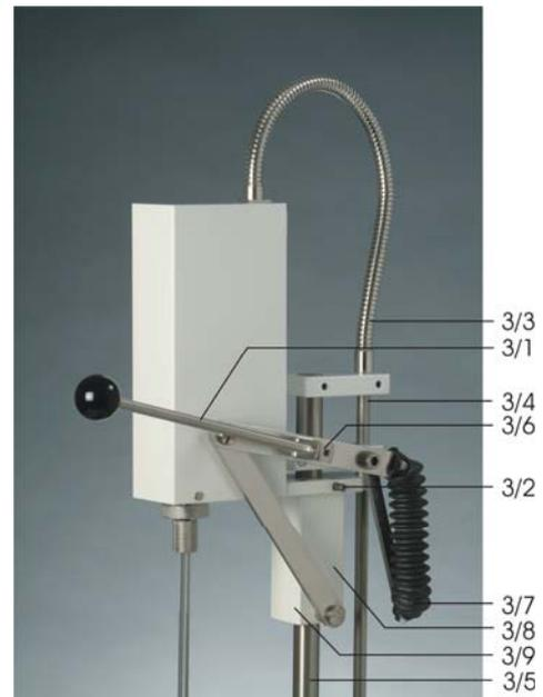
Abb. 3: Piston stroke mechanism
