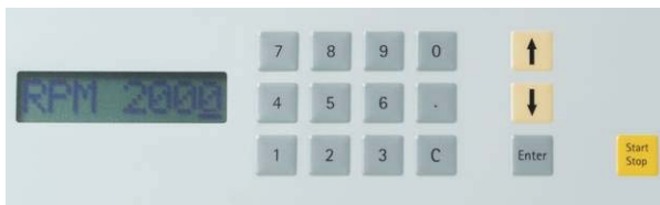
Fig. 5: Operating panel of the Mikro-Dismembrator S with key pad
