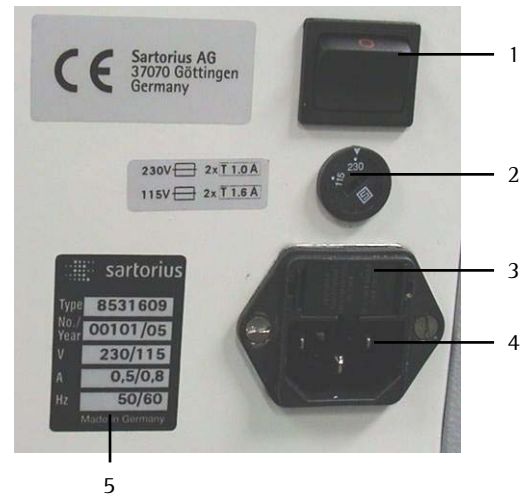
Fig. 6: Mains switch, voltage selector and fuses
