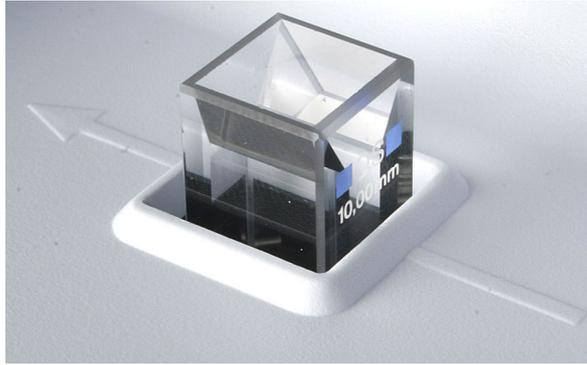
**Figure 2–5.** Aligning the measurement windows of the inserted cuvette
