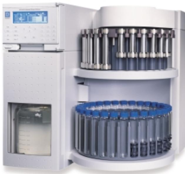
*The ASE 200 Accelerated Solvent Extractor performs extractions using less solvent and less time than traditional techniques. Two additional modules are now available to enhance the performance of the ASE 200: the Solvent Controller and AutoASE.<sup>®</sup> The Solvent Controller is an easy-to-use module that allows automated delivery of up to four solvents. AutoASE is a control and reporting application software package.*
