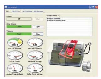
The instrument status window provides real-time monitoring of the system. In this example, the software warns that the exhaust cover door is open and flow is interrupted.
