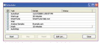
The Scheduler feature lets you create a list of tasks for the instrument to perform automatically, minimizing your involvement and maximizing workflow efficiencies.
