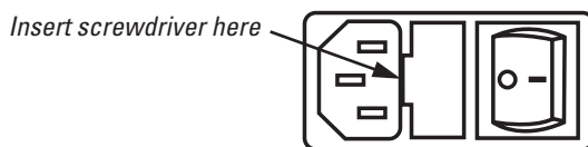
Figure 1-7. Insert screwdriver as shown to pry open the cover of the fuse holder on the power entry module.
