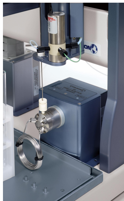
GX Direct Injection Module on the locator plate of the GX-271 ASPEC
