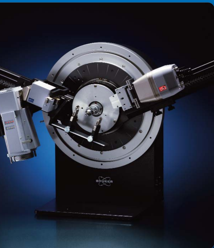
Capillary geometry with Johansson monochromator for pure K\alpha_1 radiation and VANTEC-1 detector, with unique radial Soller to reduce diffuse scattering
