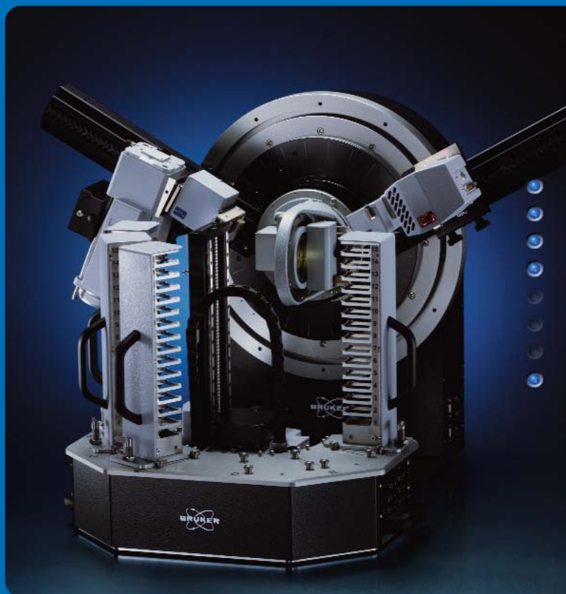
High-throughput diffraction with LYNXEYE detector and AUTO-CHANGER
