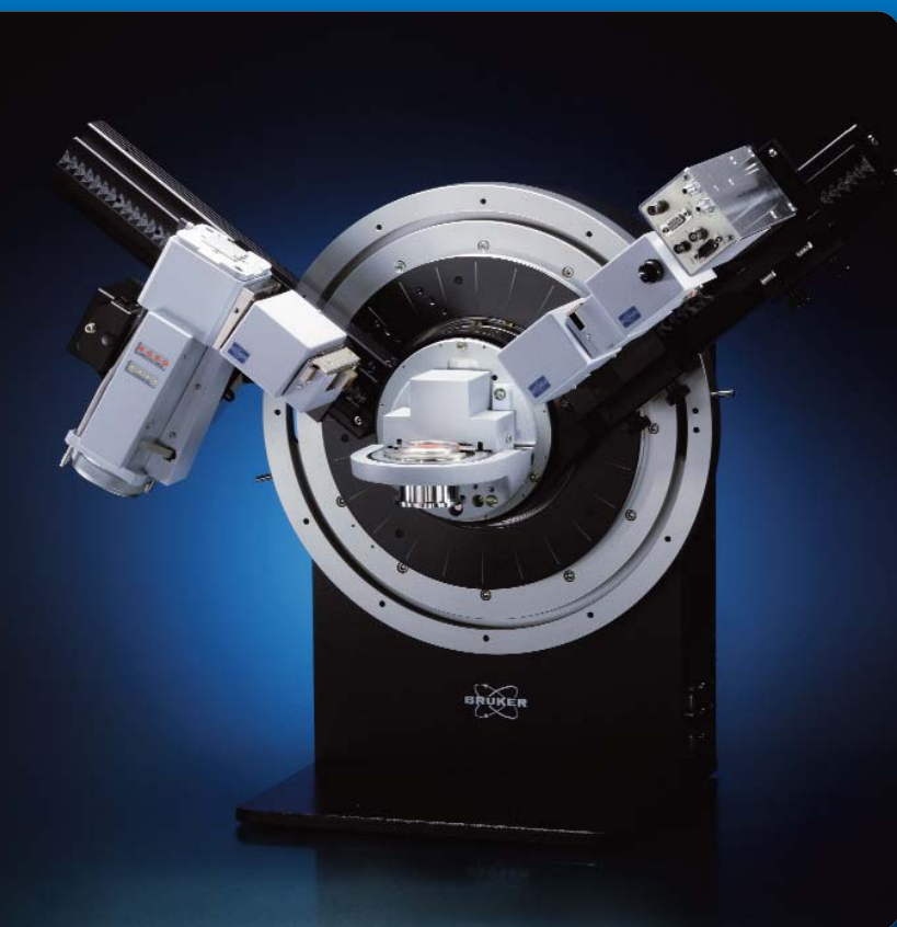
Bragg-Brentano geometry with energy-dispersive SOL-XE detector
