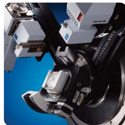
Texture setup with TWIST-TUBE
