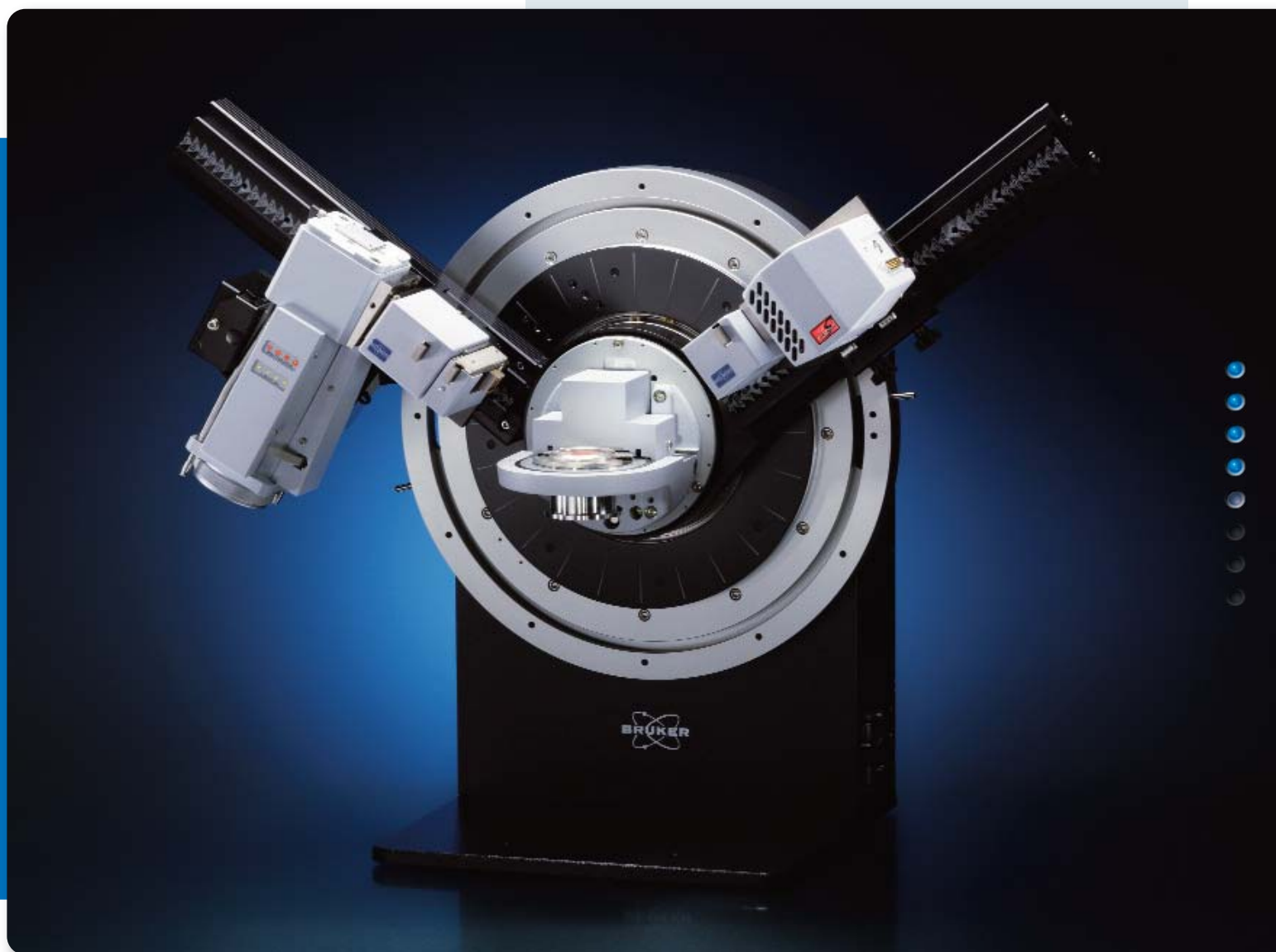
Bragg-Brentano geometry with LYNXEYE detector
