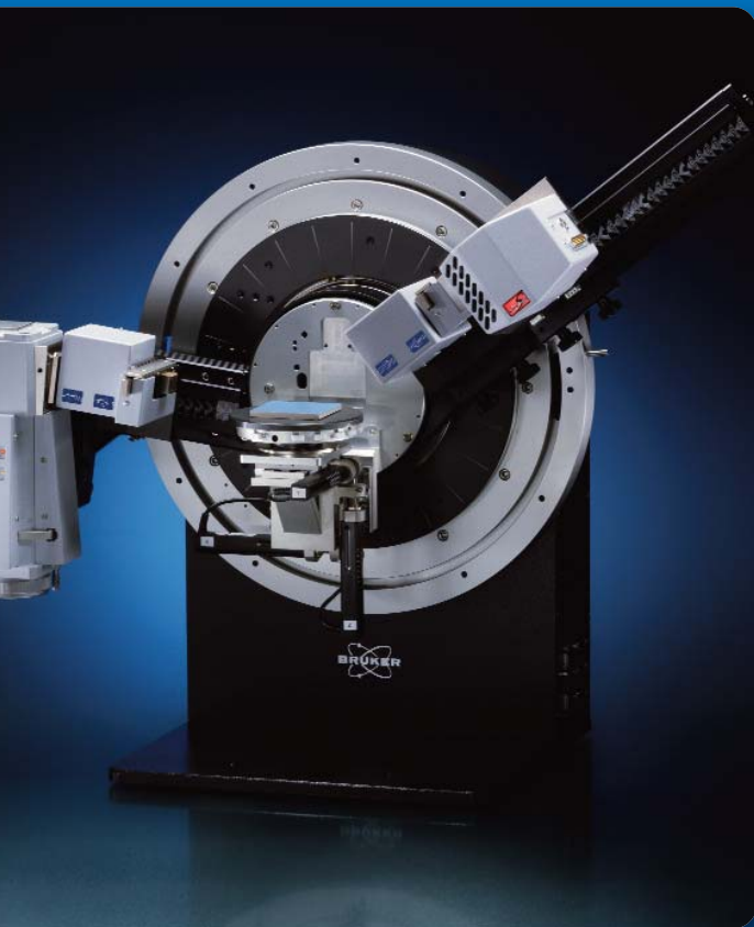
Grazing incidence diffraction TWIN/TWIN setup
