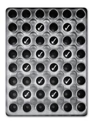
Figure 5. Wells (/) in which 0.5 ml tubes should be placed
