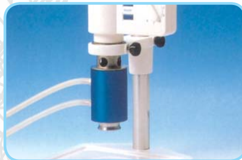
Thermal jacket When using the DIN standard or 'wide gap' coaxial cylinder configurations, the thermal jacket regulates the sample temperature
