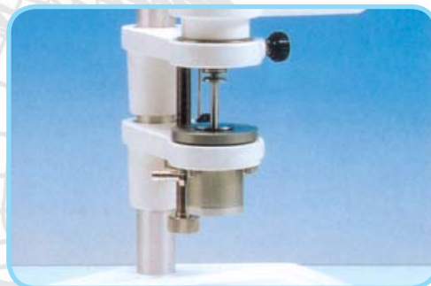
Cone and plate High viscosity fluids and pastes can be analysed with the cone and plate accessories. The Bohlin Visco 88 offers simple, accurate and repeatable gap setting whilst the integral water jacket controls sample temperature.
