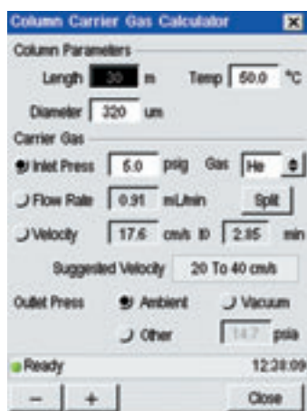
The exclusive PerkinElmer built-in flow calculator determines flow rate at a given column length and diameter.
